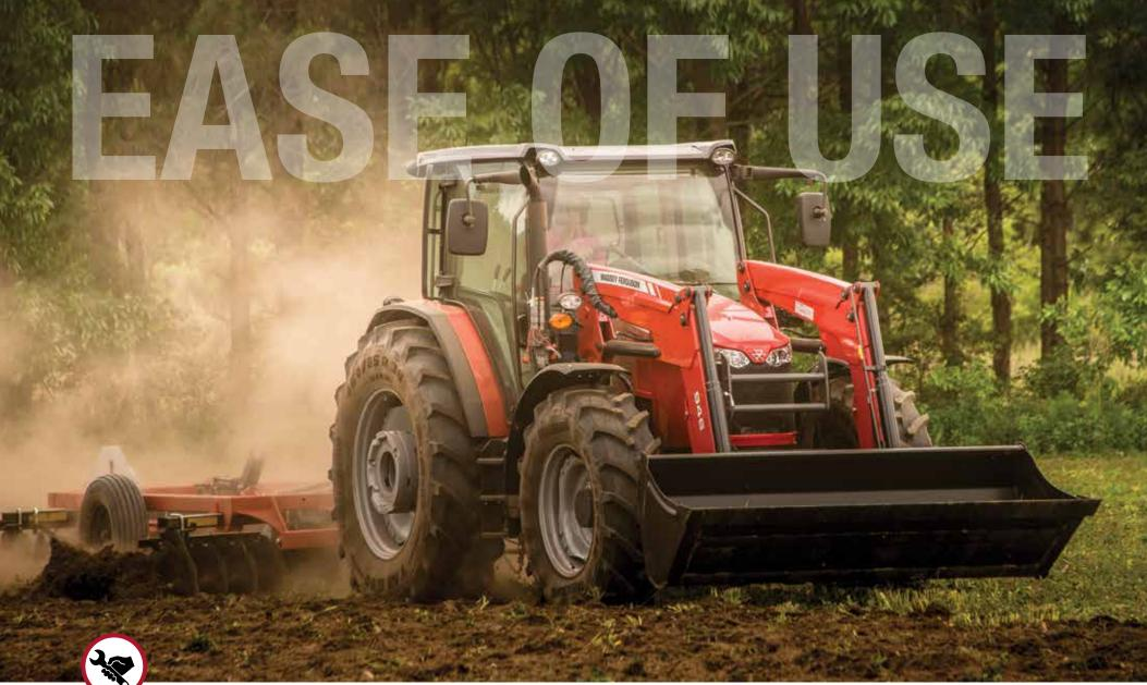
SERVICEABILITY – Whether it's access to debris screens and filters, the oil dipstick and oil fill location or the fuel tank, almost everything can be easily reached from ground level. And with a simple release latch for the hood, basic preventative maintenance takes no time at all.
